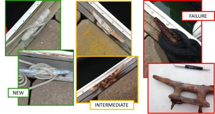
Cleat Damage Estimate
